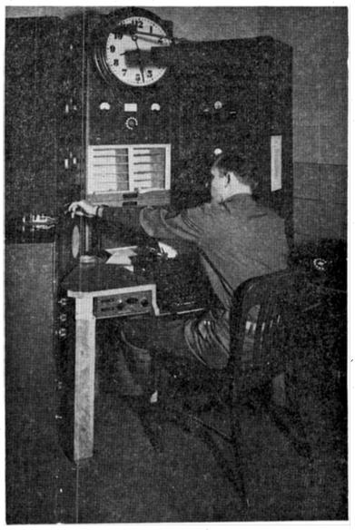
ARMY AIRWAYS COMMUNICATION STATION—This station maintains point to point contact between air fields and also contact with planes while they are in flight.
