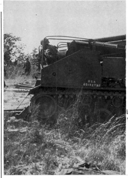
THE M-41S OF THE 999TH, SHOWN HERE, HAVE A MAXIMUM RANGE OF 16,350 YARDS. DEVELOPED DURING WORLD WAR II, THEY WEIGH 42,000 POUNDS, CAN MOVE AT 45 MILES AN HOUR, CARRY 32 ROUNDS OF AMMUNITION AND CAN FIRE AT THE RATE OF THREE
